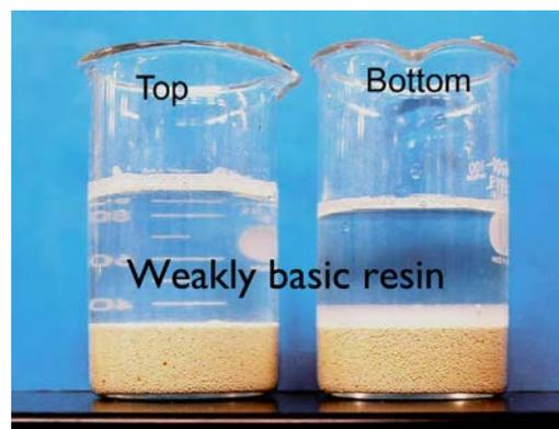
Most demineralizers that use weak base anion resins for water treatment also use strong base anion resins. In order to minimize the amount of caustic used to regenerate the resins, a technique known as thoroughfare regeneration is generally used. Thoroughfare regeneration is the use of waste caustic from the SBA vessel to regenerate the WBA resin (see the corresponding Tech Fact).
